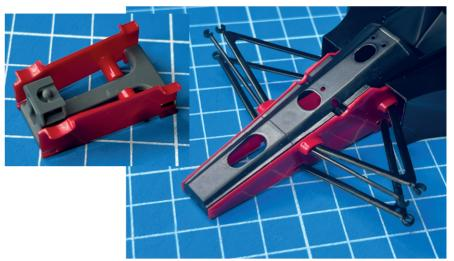
Cut the suspension kit parts as shown to insert them into the jig.
